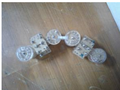
Figure 3: Two rigid spine segment connected by a flexible strip
